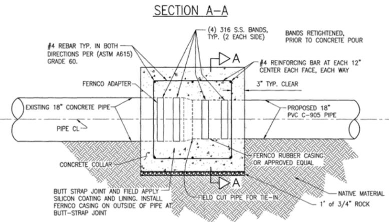
CONSTRUCT 826.24' L.F. OF 18" PVC C-905 IRRIGATION PIPE
